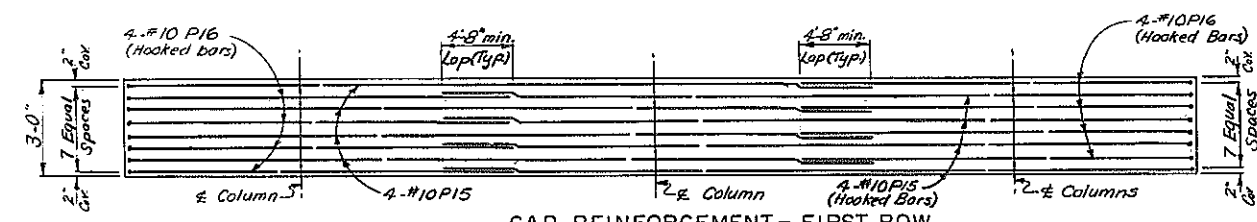
CAP REINFORCEMENT- FIRST ROW
