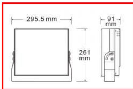
**INEX-TECH's** LED strobes provide a very powerful illumination, or Flashlight, source for Intelligent Traffic monitoring solutions such as ANPR (automatic number plate recognition), Red Light Violation, Open Road Tolling and Weigh-in Motion systems. Utilizing the latest high power LED technology available, the IZ-SW2 illuminators series is fully integrated with internal timing, intensity control, trigger input and long distance communications.
