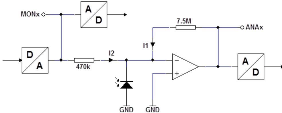
The drawing above is a simple circuit diagram of one channel. When the photodiode is illuminated with light from the sensor it proportionally sinks a current to the incoming light power. This causes the output of the OPAMP to go high so the current is supplied across the 7.5 M $\Omega$  resistor. When the light becomes too bright the OPAMP output is clipped, and the controller supplies additional current via the DAC and the 470 k resistor until the OPAMP output is "unclipped."
