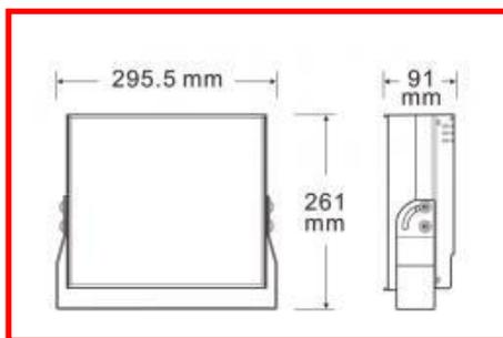
**INEX-TECH's** LED strobes provide a very powerful illumination, or Flashlight, source for Intelligent Traffic monitoring solutions such as ANPR (automatic number plate recognition), Red Light Violation, Open Road Tolling and Weigh-in Motion systems. Utilizing the latest high power LED technology available, the IZ-S2 illuminators series is fully integrated with internal timing, intensity control, trigger input and long distance communications.
