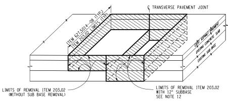
FULL DEPTH AND JOINT REPAIR DETAIL (TYP.)
