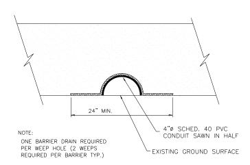
SECTION C-C BARRIER WEEP HOLE DRAIN DETAIL
