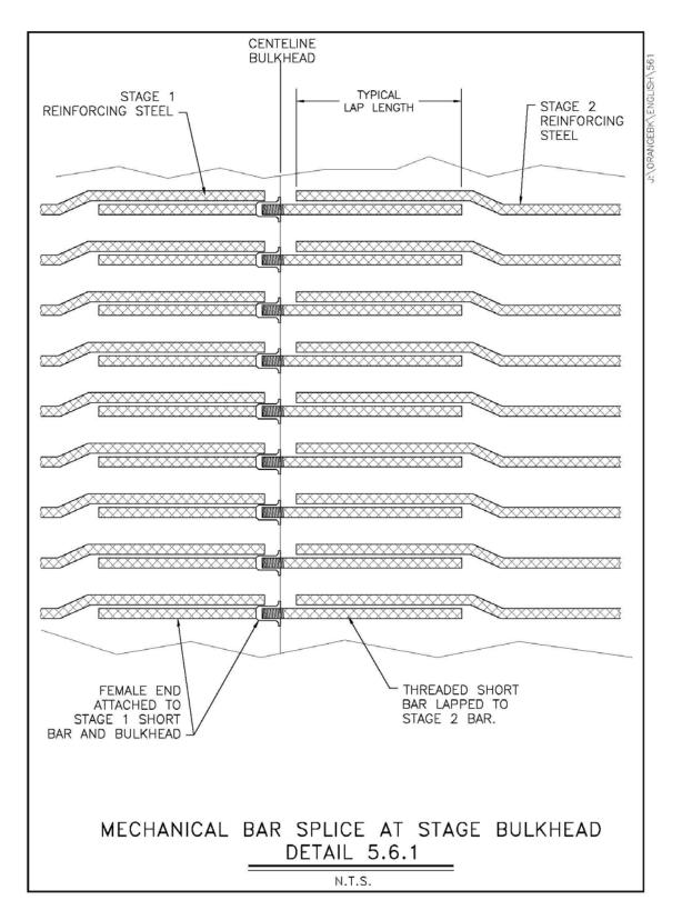
When stage construction is required, splicing of the transverse bars shall be within a closure pour between adjacent beams. A closure pour should never be directly over a beam. Where room is limited between stages, mechanical bar splices should be used as described in Subsection 5.6.1.
