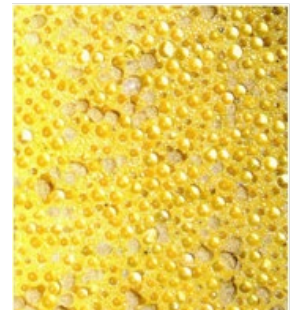
Exhibit 19: Closeup of Recess Triple Drop Pavement Marking, with Glass Beads and Ceramic Elements
